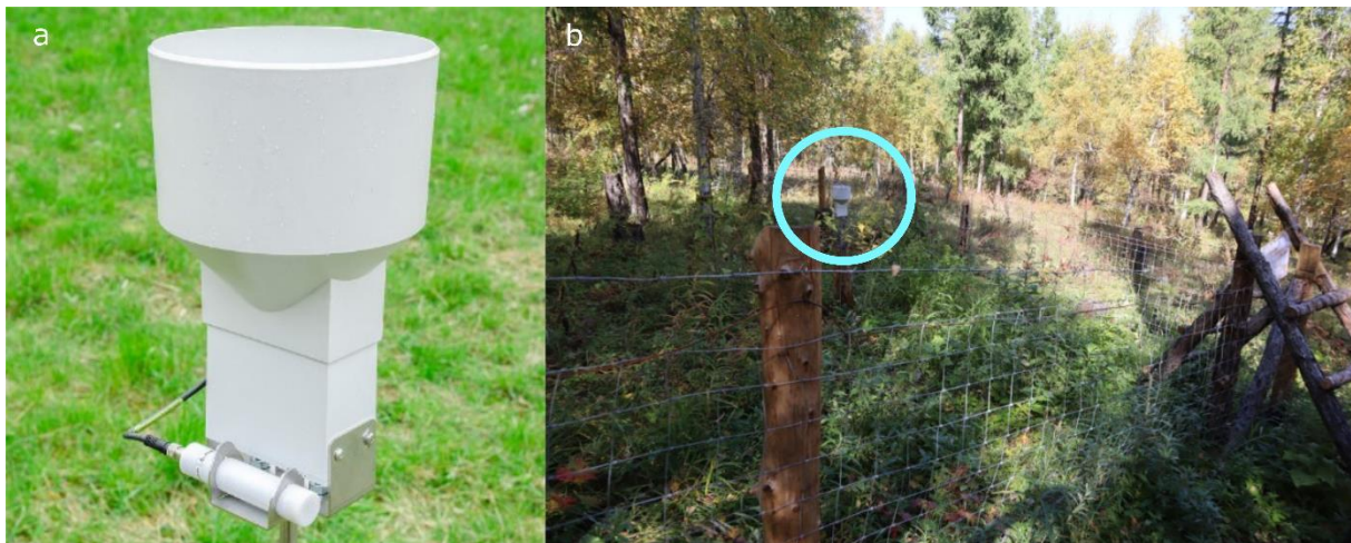
Figure 5. a = Pronamic Pro rain gauge (EMS Brno, 2024), b = rain gauge placement at the Tunkhel demonstration plot E1.
