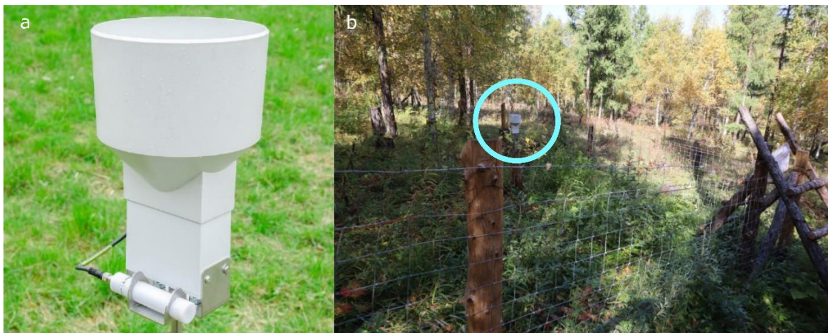
Figure 12. a = Pronamic Pro rain gauge (EMS Brno, 2024), b = rain gauge placement in the Tunkhel demonstration plot.
